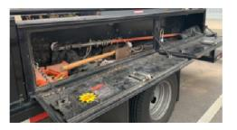
**4.28.12.3 CUSTOM EXPANDED METAL BOX:** On top of side compartment in 4.28.2a shall be a custom metal box that is the same depth as toolboxes, 8" tall plus solid metal lid, and is the length of the body compartment. Opening shall have a hinge at the bottom and be lockable from the top with a keyed lock.
